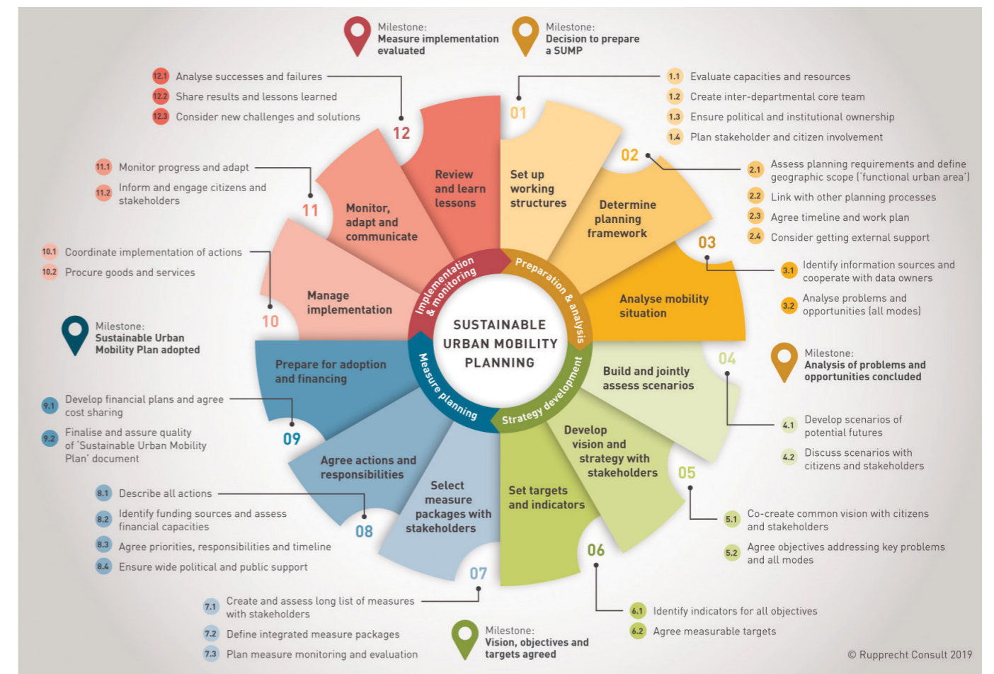
Figure 15: The SUMP cycle and its different phases (= four quadrants) and steps (12 = segments). © Rupprecht Consult.
